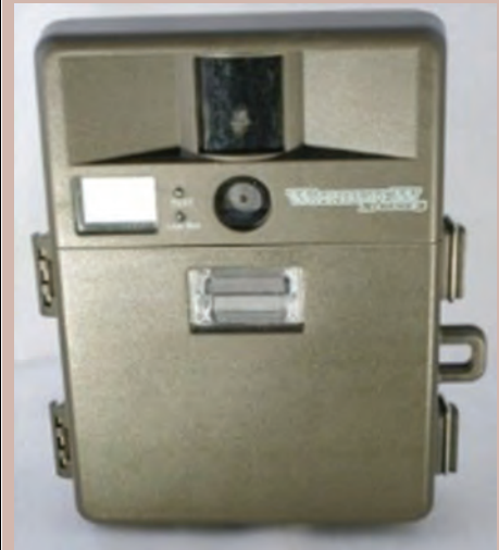
Top: A camera trap with motion detector on top, lens in the middle and flash on the bottom Top Left: a Sumatran tiger caught on the camera (it destroyed three camera traps in one weekend)
